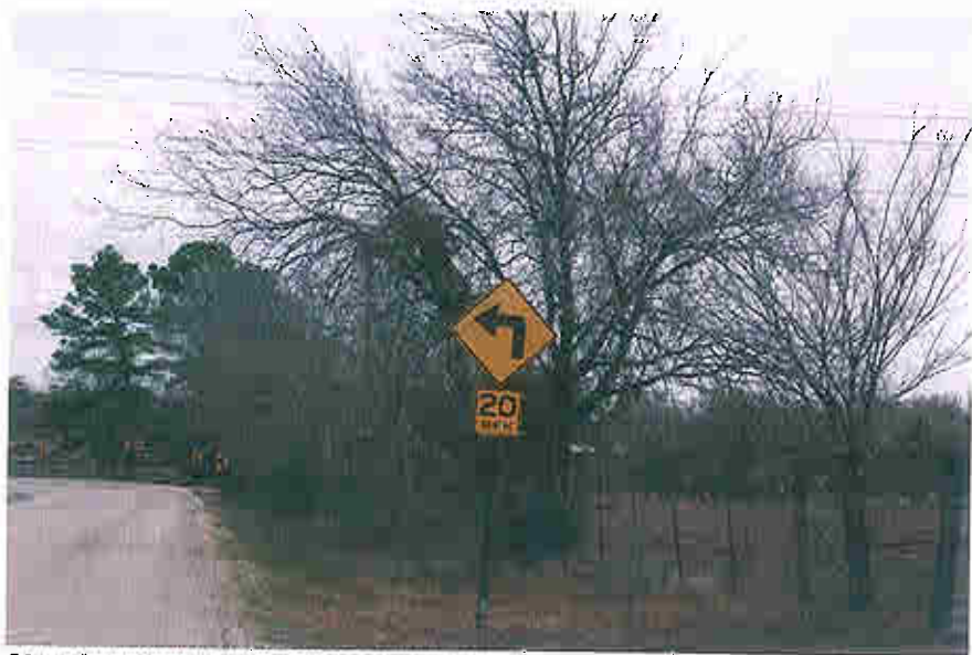
A turn sign provides drivers advance warning of a change in the alignment.
