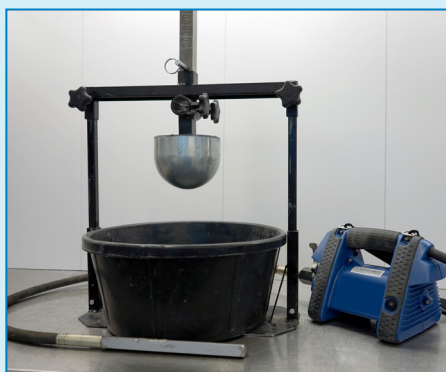
The V-Kelly evaluates concrete workability by measuring the rate that a steel mass penetrates into concrete as it is vibrated.
