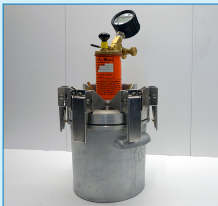
The Super Air Meter® evaluates concrete freeze-thaw durability by measuring the air system and distribution of air in fresh concrete.
