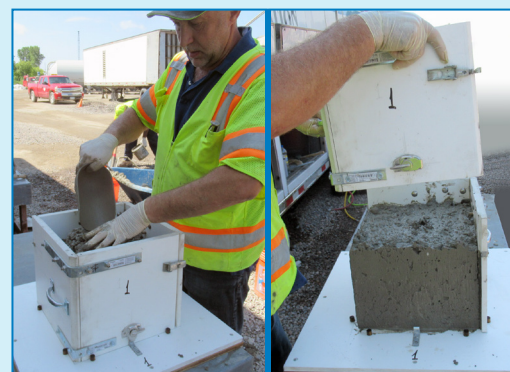
The Box Test is used to assess the workability of slip formed concrete mixtures. In the photos above, a sample is being prepared for assessment.
